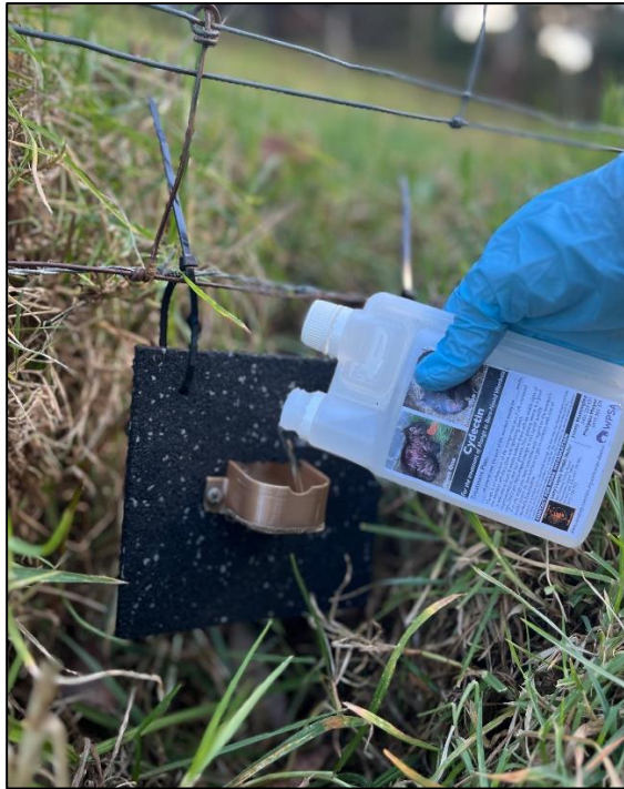
Burrow flap with 3D moulded insert to hold Cydectin is attached using pop rivets.
