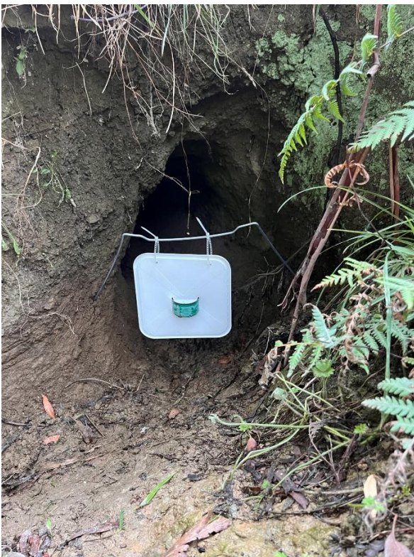
Wire frame can be expanded and pushed into sides of burrow depending on it's shape.
