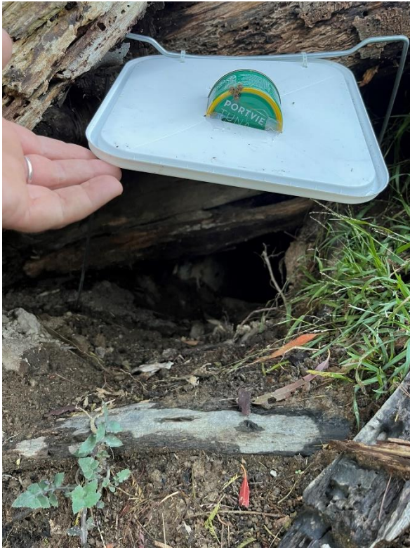
Showing plastic flap with tin inserted able to swing back and forth.
